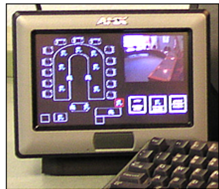
A small touch-screen easily selects one of 30 pre-selected camera shots or simple controls for a quick pan/tilt/zoom.
